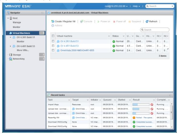
**10.** When the installation is complete (indicated by all three files showing "Completed Successfully" in the Result column of the Recent tasks table), click on **Virtual Machines** in the
