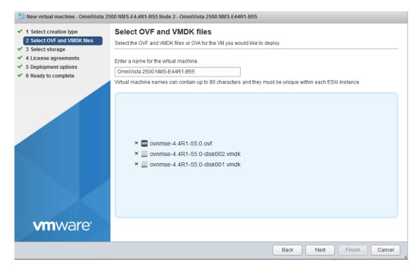
**5.** Enter a name for the VM (e.g., OmniVista 2500 NMS-E44R1-B55, click to locate and select the downloaded installation files (or drag the files into the window), then click **Next**. Note that if you plan on configuring a High-Availability installation, you could add Node information to the name (e.g., OmniVista 2500 NMS-E44R1-B55 Node 1) to more easily identify the VM.
