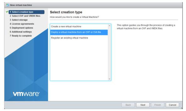
4. Select Deploy a virtual machine from an OVF or OVA file and click Next.
