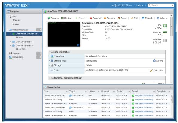
**11.** Click on **Console** at the top of the screen and select **Open Browser Console** to open a Console and go to <u>Completing the OmniVista Installation</u> to complete the installation.
