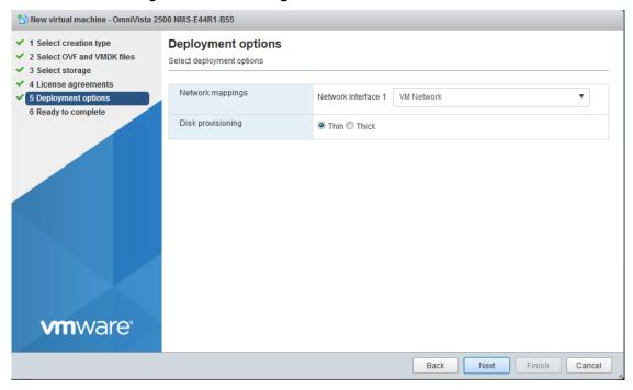
**8.** In the **Network mapping** field, select the Destination network that the deployed VM will use. In the **Disk provisioning** field, select **Thin**. Click **Next**.
