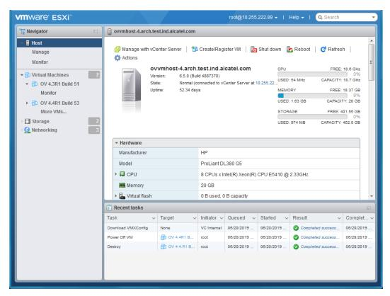
**3.** Select the Host on which you want to install OV 2500 NMS-E 4.4R1 and click on **Create/Register VM**. The first screen of the New Virtual Machine Wizard appears.
